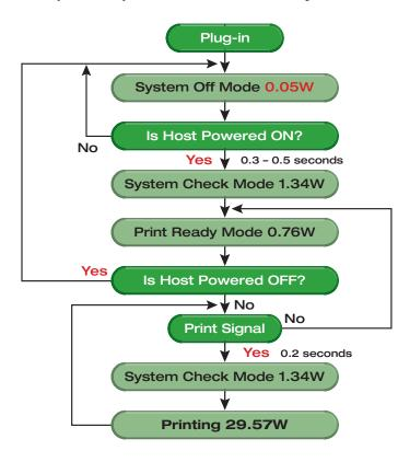
Those clever engineers at Star have designed this printer to correspond directly to the PC it has been attached to. Users will first of all notice that there is no power switch and that the printer can only be turned on by actually attaching the included USB cable to the printer and PC / terminal. The printer will only activate when the PC / terminal is powered up otherwise it can remain in standby mode, thus saving power.
